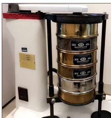
Figure 20: Ro-tap sieve shaker for particle size distribution
