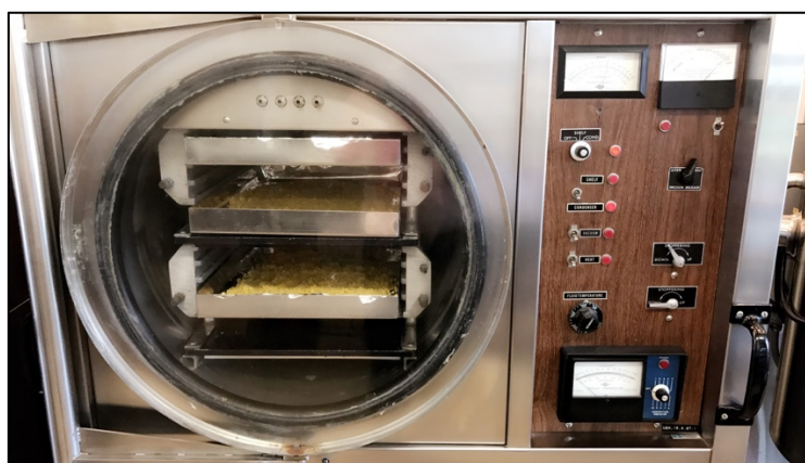
Figure 9: Bulk freeze dryer (Make: Virtis Inc.)
