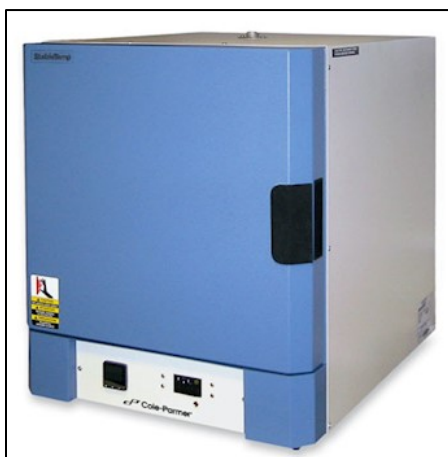
Figure 14: Muffle furnace by Cole Parmer (Model: Box furnace, 51800 series)
