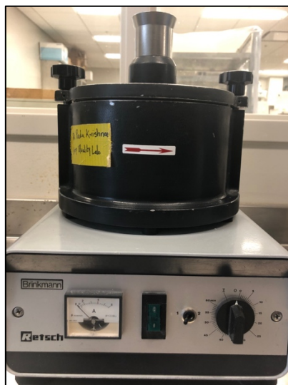
Figure 10: Retsch mill (Make: Retsch Brinkmann, high speed rotor mill)
