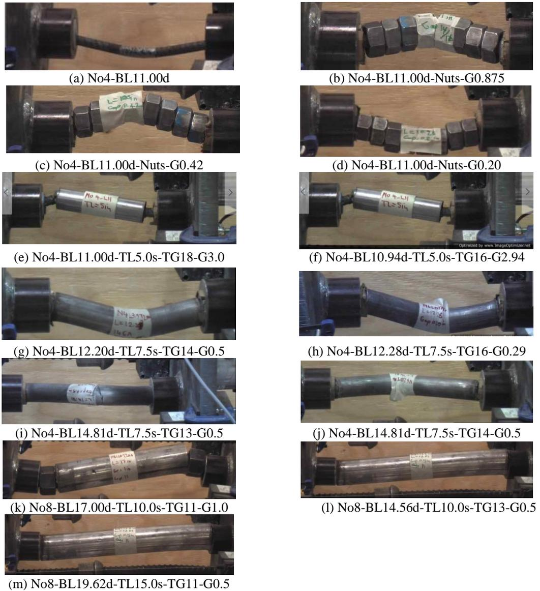
**Figure 2.22 – Failure modes for BRR specimens tested by Boudaqa et al. (2016)**
