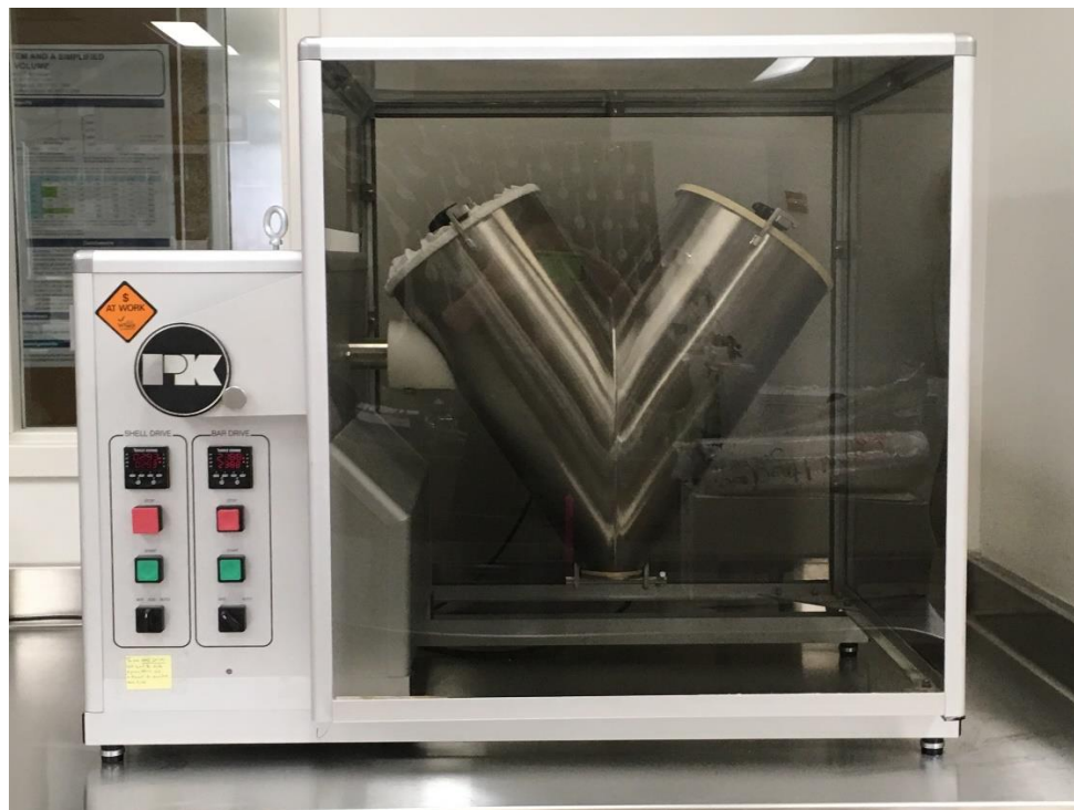
Figure 5. V-shaped lab scale blender (Patterson-Kelley, Harsco, East Stroudsburg, PA) for uniform and homogenous distribution of enrichment ingredients within flour.
