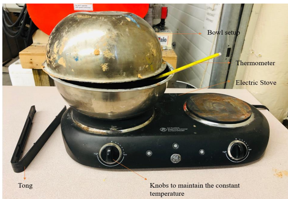
Figure 8. 100% Humidity experimental set up
