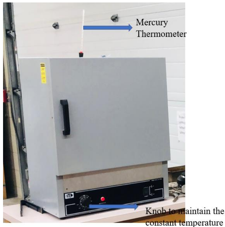
Figure 9. Non-vacuum electric oven with thermometer and knob locations
