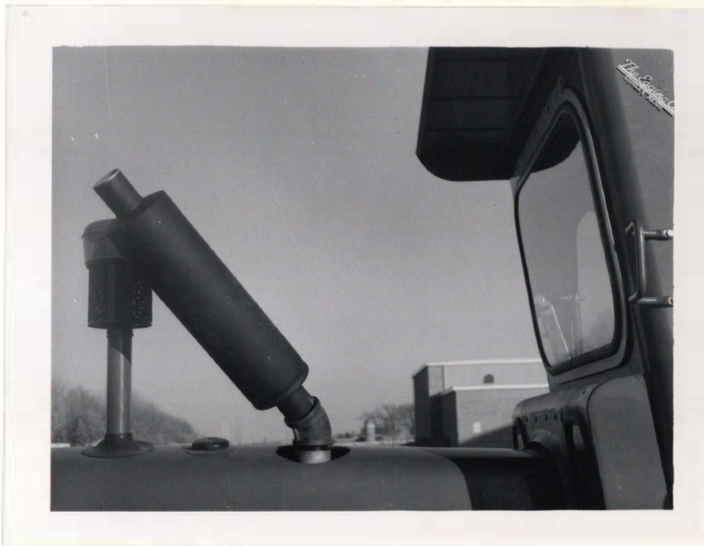
Figure 6. Factory Replacement Muffler at a 45° Angle
