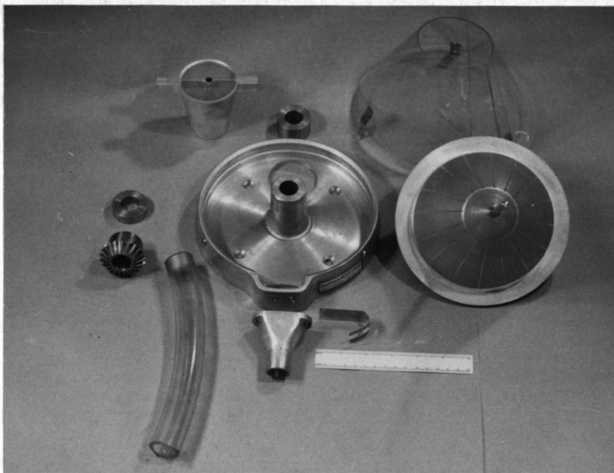
Figure VII. Cone Meter, Left to Right and Bottom to Top: Delivery Tube, Drive Gear, Bushing, Loader, Discharge Funnel, Cone Base, Bushing, 6-inch Scale, Deflector, Cone with Base Plate and Windshield
