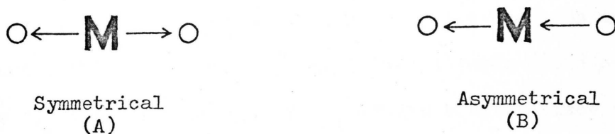
Figure VII. Trans Metal-Oxygen Stretching Modes. The symmetrical mode is infrared inactive and the asymmetrical mode is infrared active. M is any metal which forms a dioxo- species.
