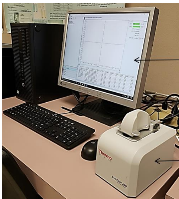
Figure 5. 3 Nanodrop 2000 spectrophotometer used for estimating protein content of the dialyzed CFE with the help of NanoDrop2000 software
