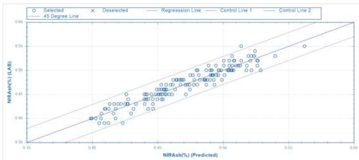
Figure 14. Correlation plot between NIRS method and reference analysis method of NIR ash % with combined 2018/2019 calibration dataset(N=155)
