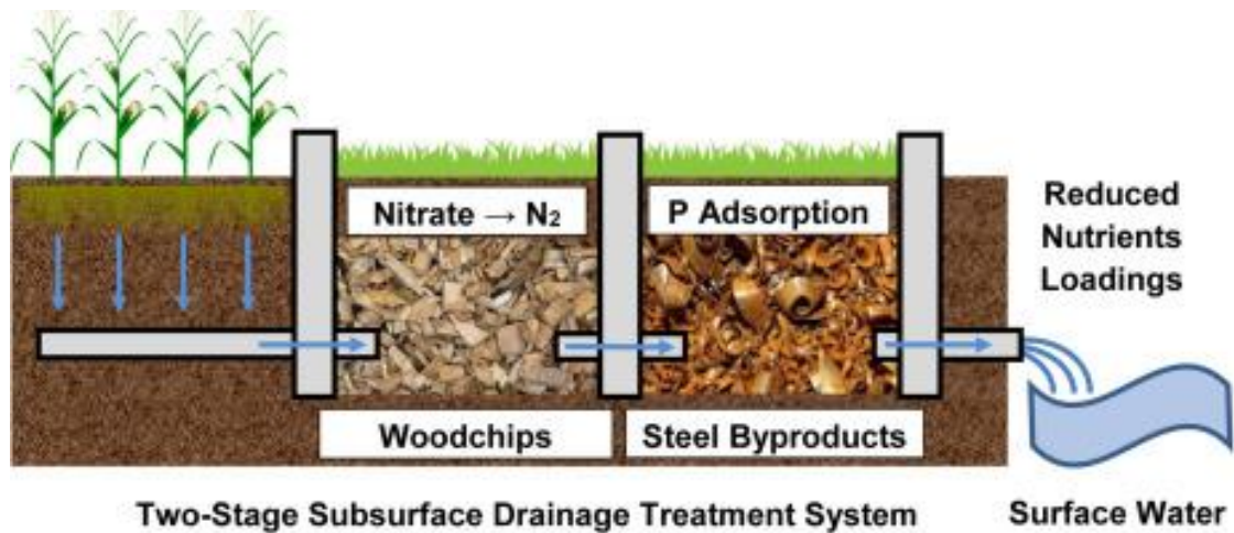
Figure 5: Typical woodchip bioreactor for denitrification and improving water quality. Reproduced from Hua et al. 2016, and https://www.egr.msu.edu/bae/water/woodchip-bioreactor .
