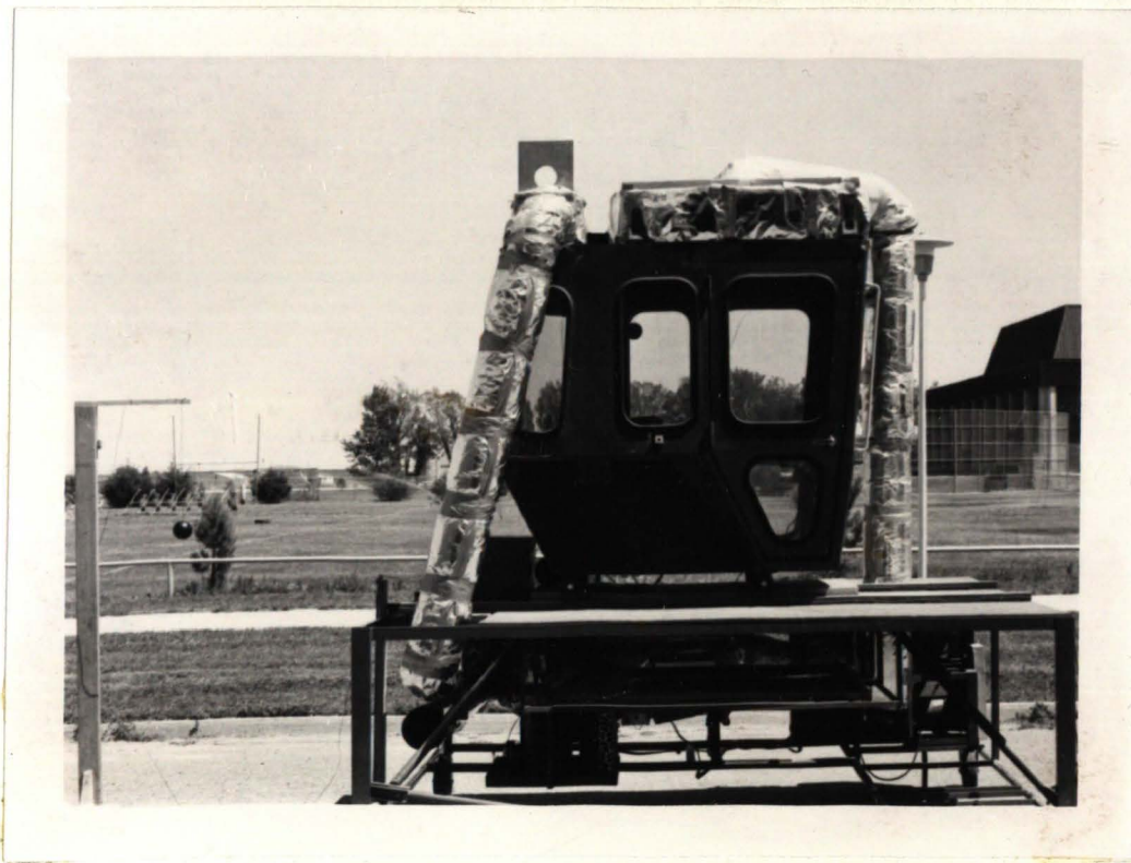
Figure 5. Tractor Cab Ductwork and Outside Black Globe
