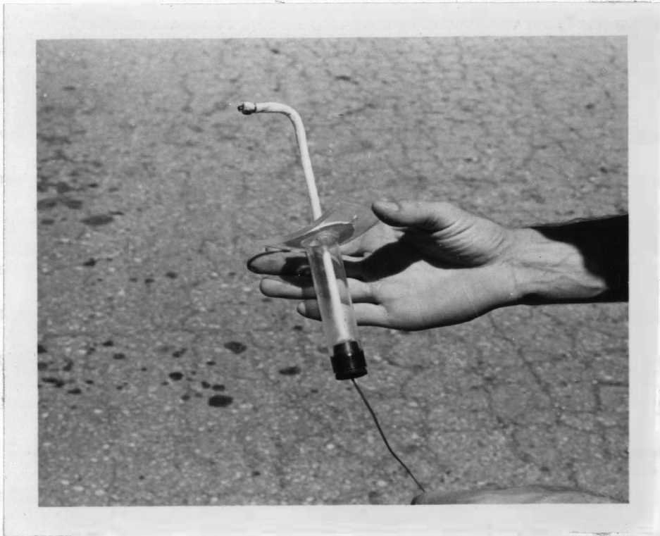
Figure 11. Temperature-Humidity Device for Duct Q0.
