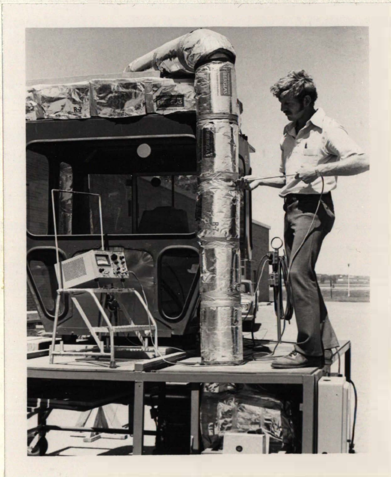
Figure 7. Taking Air Velocity Readings in Inlet Duct
