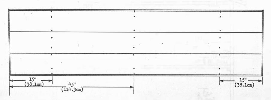
Figure 11. The 24 locations where air velocities and patterns were obtained. Top view
