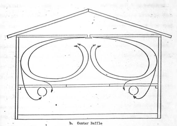
Figure 18. Air flow patterns comparing side and center baffles for slotted pipe under-slat ventilator.
