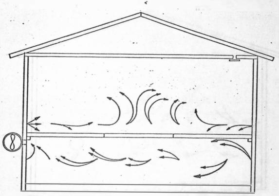
Figure 23. Air flow patterns for outside wall pit ventilator system, side baffle, center location.
