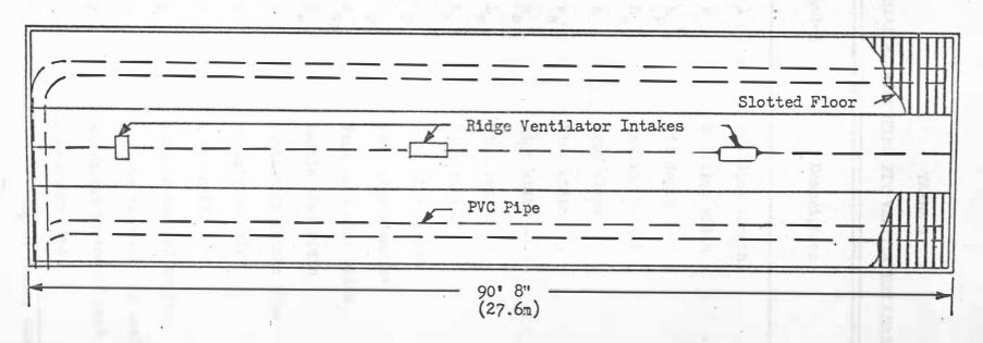
Figure 2. Floor plan, prototype swine finishing unit.
