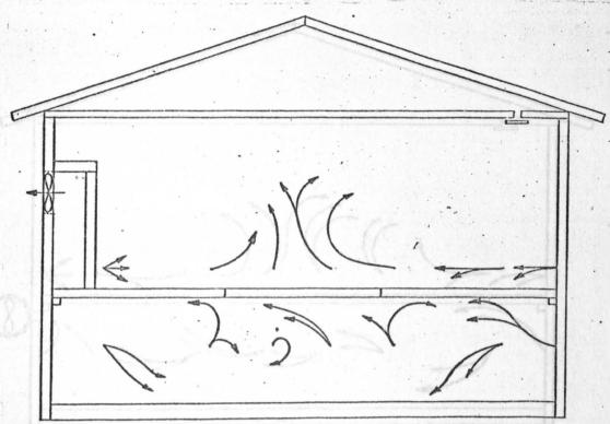
Figure 21. Air flow patterns for hooded manure pit exhaust system, center location.
