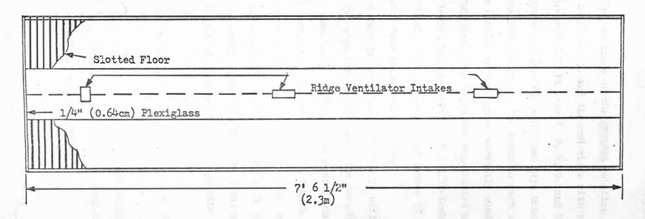
Figure 4. Floor plan, model swine finishing unit.
