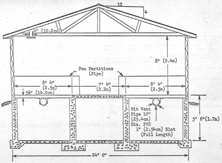
Figure 1. Front view, prototype swine finishing unit.
