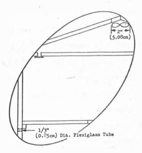
The last system (Figure 10), a pressurized pit ventilator, forced air below the slats through 18 1/3-inch (0.85 cm), plexiglass tubes spaced uniformly on each side of the model. Air was introduced into the attic through two 2-inch (5.27) I. D. PVC tubes.
