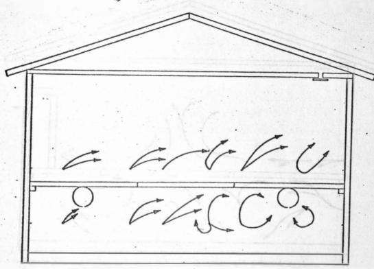
Figure 19. Air flow patterns for slotted pipe under-slat ventilator, center location.
