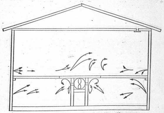
Figure 20. Air flow patterns for centered duct pit ventilator, center location.
