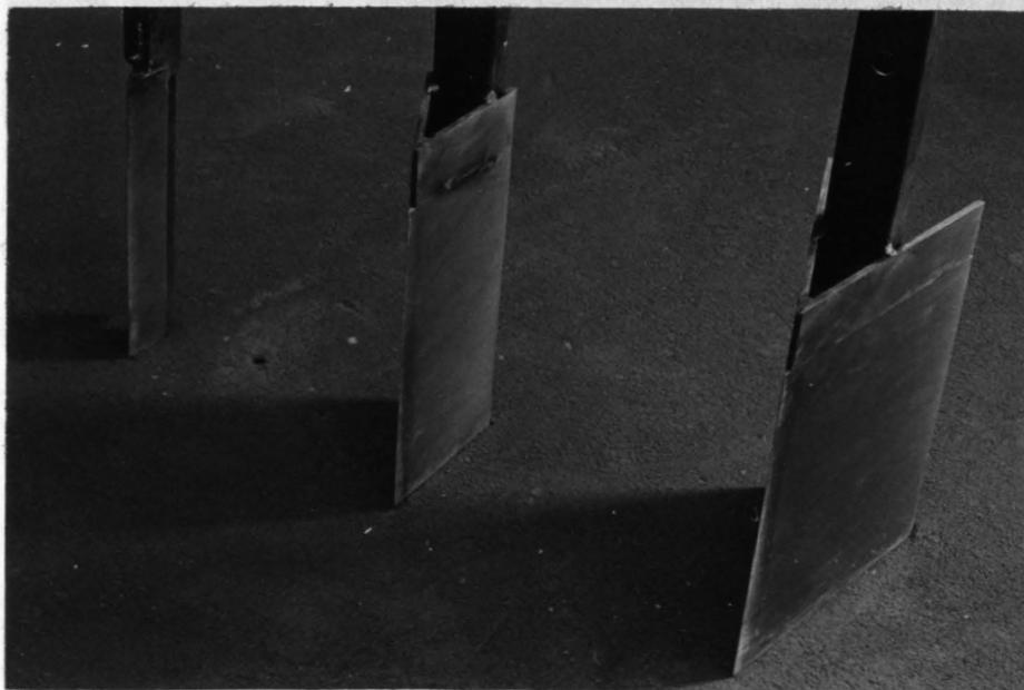
Figure 2. Model chisels
