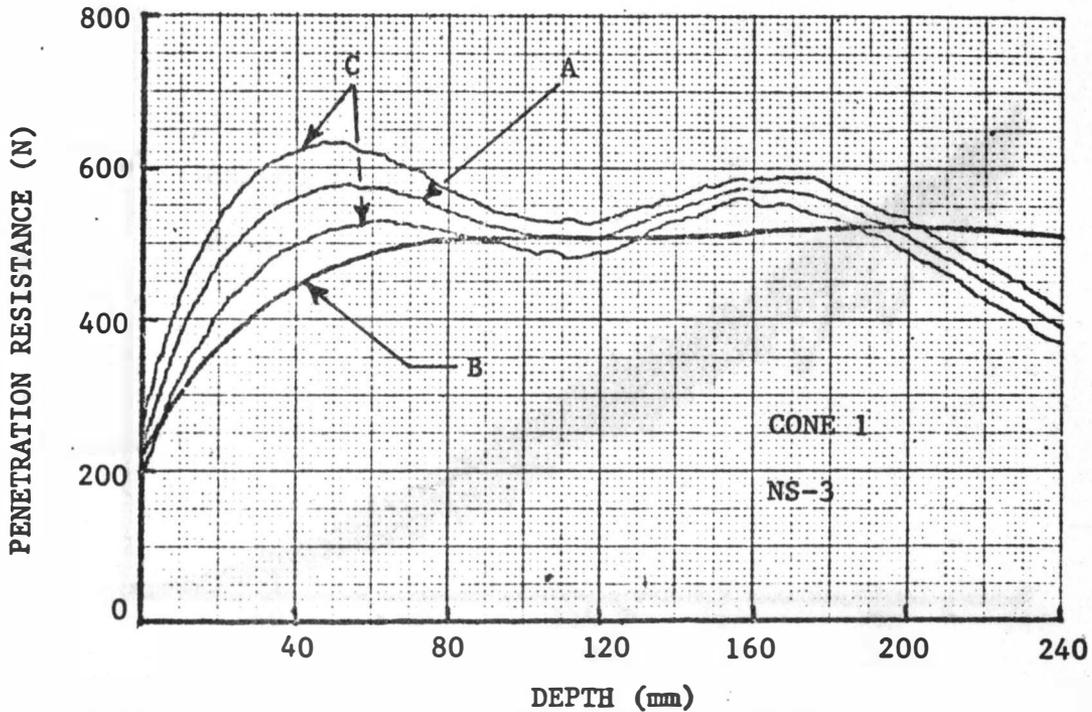
Figure 23. Cone penetrometer data curves for cone 1, NS-3, (A) cone penetrometer data, (B) running average, (C) error band of one standard deviation
