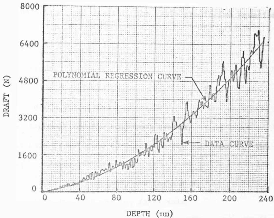
Figure 12. Data and polynomial regression curves for chisel 3, NS-2
