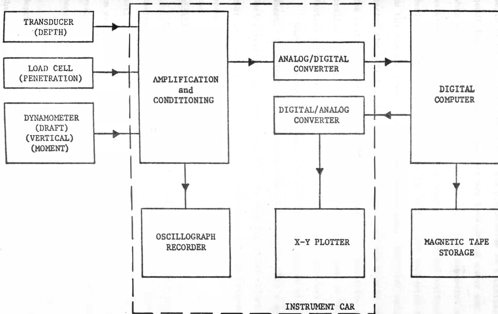
Figure 10. Schematic diagram of instrumentation systems
