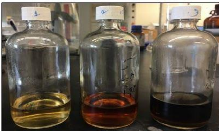
Figure 4.3. Extraction of lignin from biomass at different temperatures.
