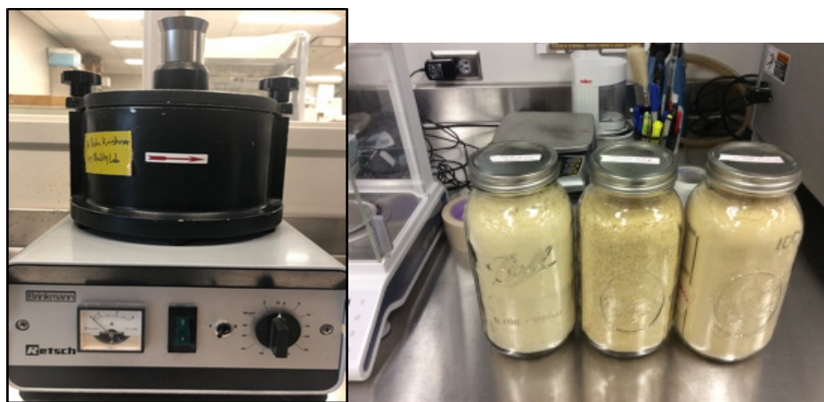
Figure 10. Dry grinding of DDG using Retsch mill employing a 0.2- and a 0.5-mm sieve. Retsch mill (Retsch Brinkmann, GmbH & Co.KG, 5657 HAAN1, and Germany)
