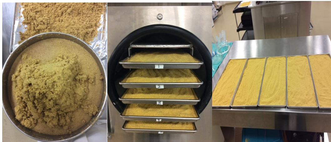
Figure 9. Technique for Washing, Freeze Drying and Sterilization of DDG
