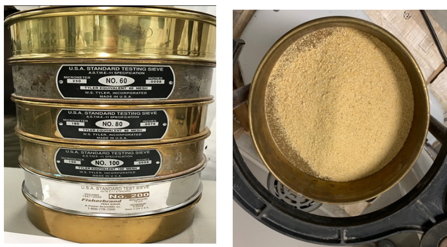
Figure 11. Stacked Tyler Sieves for determination of particle size distribution
