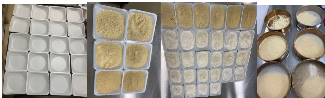
Figure 12. Processes used in determining particle size distribution of flour samples
