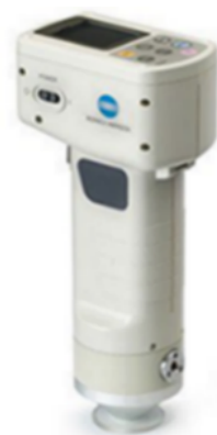
Figure 14. Calorimeter - Konica Minolta CR-400 chromameter (Image ethanol plant fractions)
