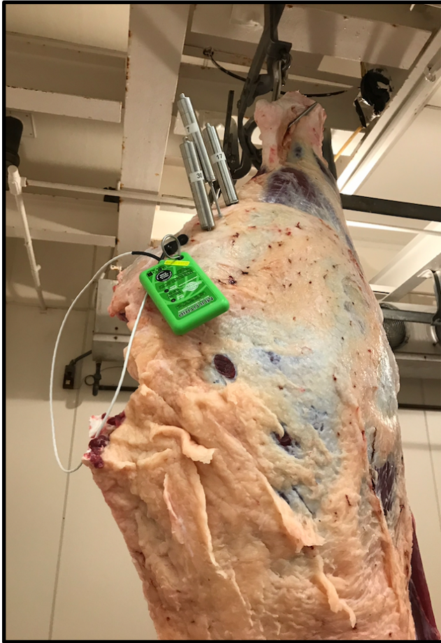
Figure 2.2. Temperature data loggers were placed in the center of the round in the 20-, 15-, 10-, and 5-cm position.
