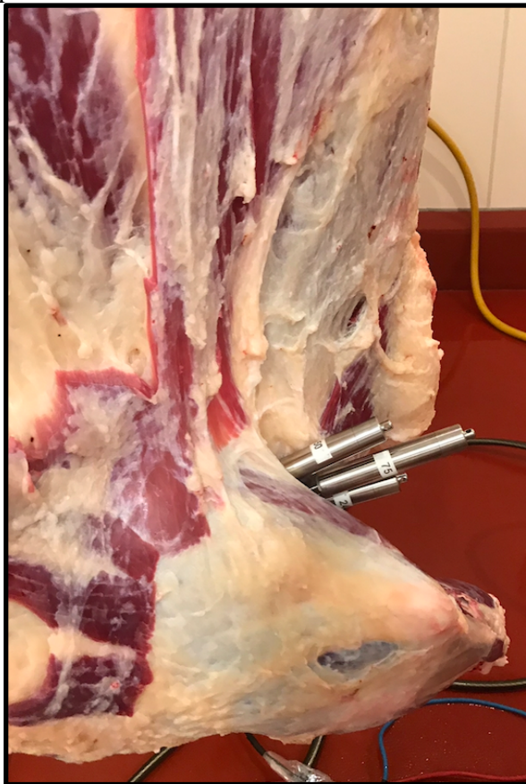
Figure 2.3. Temperature data loggers were placed in the chuck immediately posterior to the foreleg in the pocket between the brisket and the chuck in the 20-, 15-, and 10-cm position.
