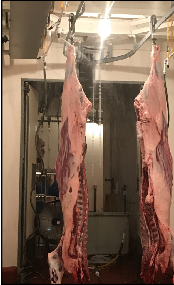
Figure 2.1. Two section spray chilling system suspended above beef sides spraying water during chilling period.
