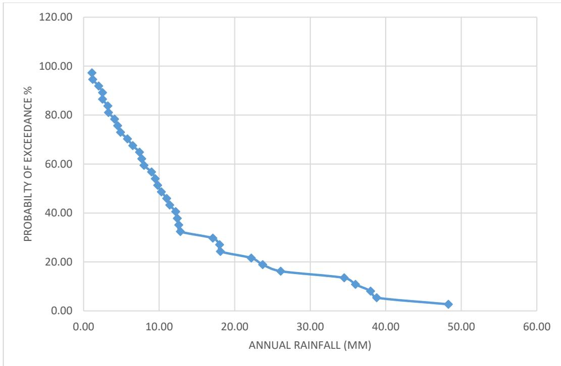
Figure 4.12 Probability plot of the total annual rainfall for Wadi by using linear scales for both axes.
