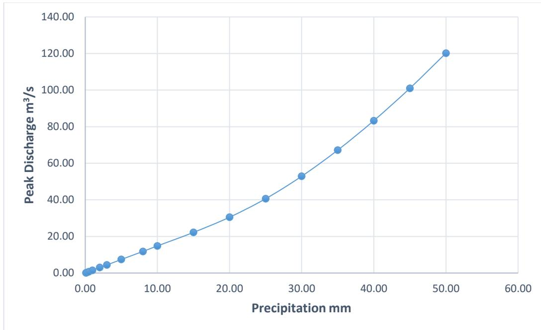
Figure 4.8 Peak discharge interacting with precipitation over Wadi Abu Nashayfah.
