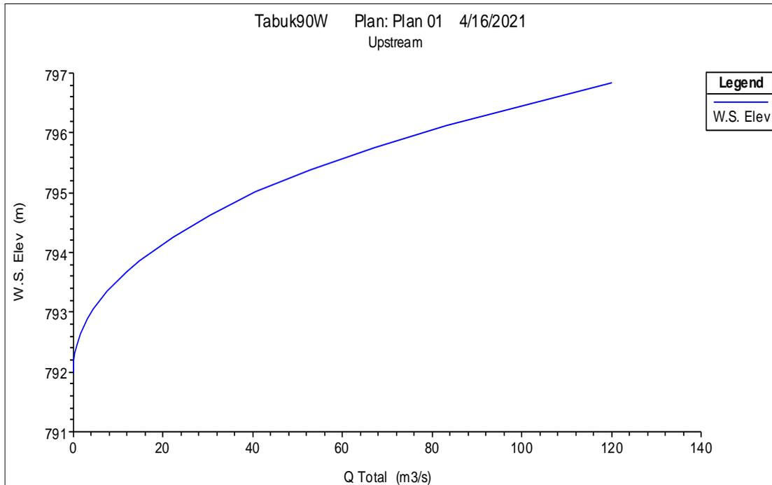
Figure 4.9 Water surface corresponding to peak discharge for section 1.
