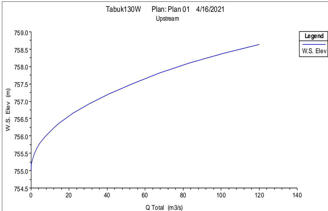
Figure 4.10 Water surface corresponding to peak discharge for section 2.
