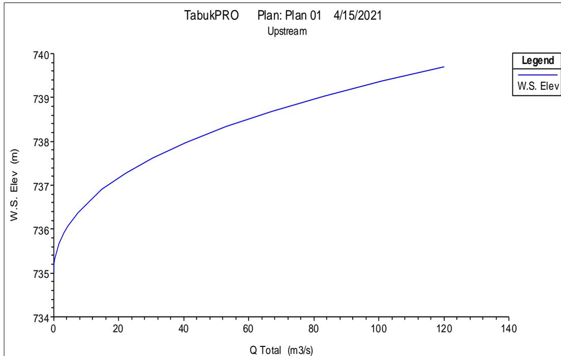
Figure 4.11 Water surface corresponding to peak discharge for section 3.
