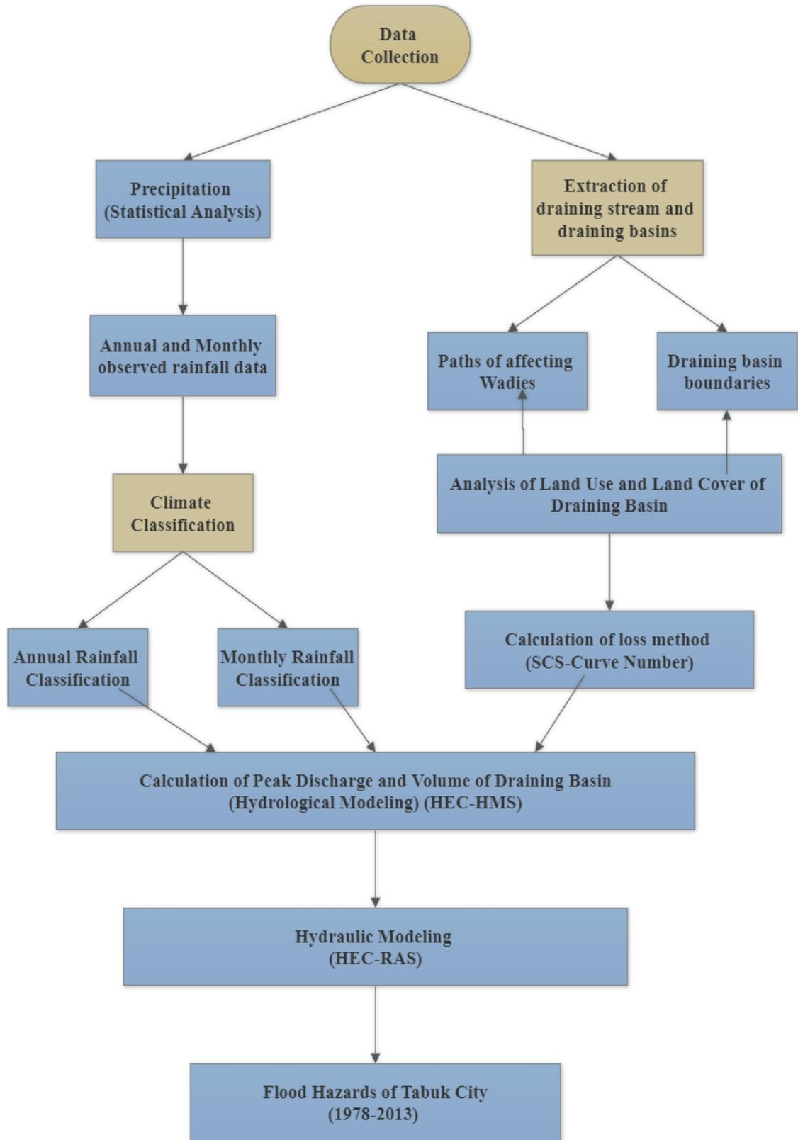
Figure 4.7 Flowchart showing the process applied in this study.
