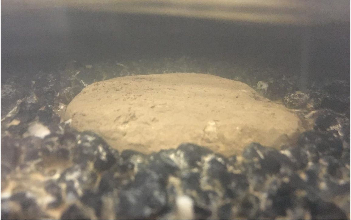
Figure 4.15 About 1-hour after start of erosion test
