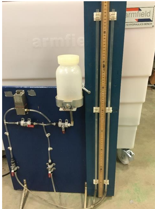
Figure A.3 Static Manometer set up
