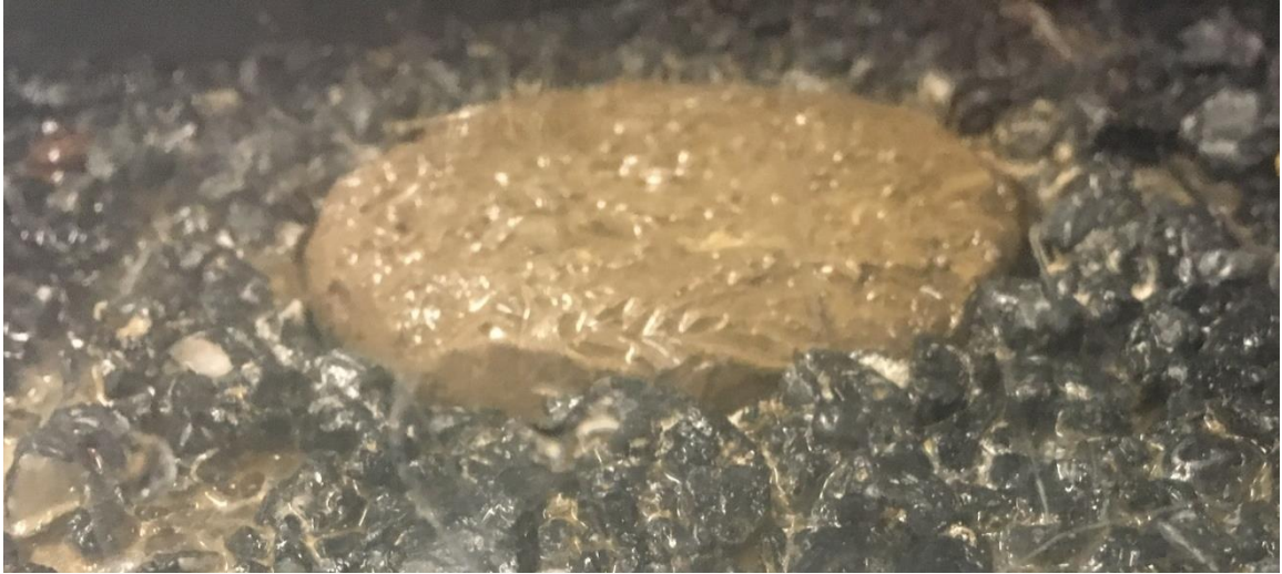
Figure 4.24 Example of little-to-no Erosion
