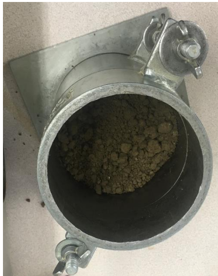
Figure 3.4 Layer of soil before being compacted
