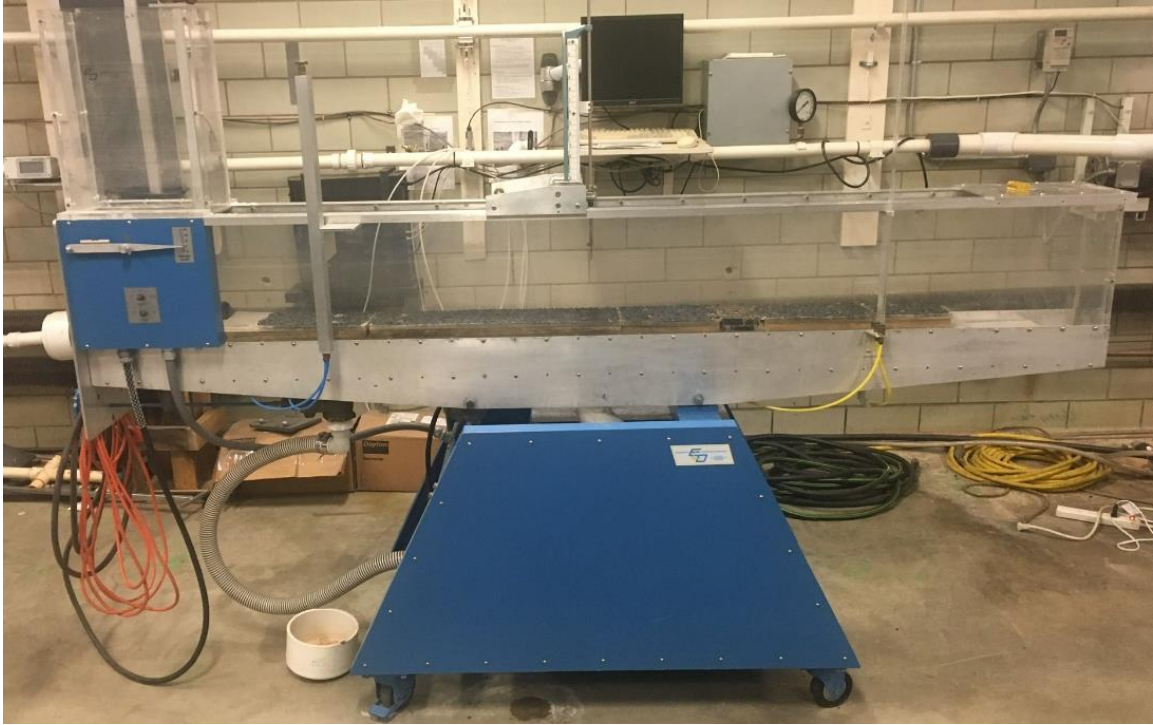
Figure 4.1 A-8 Hydraulic Channel
